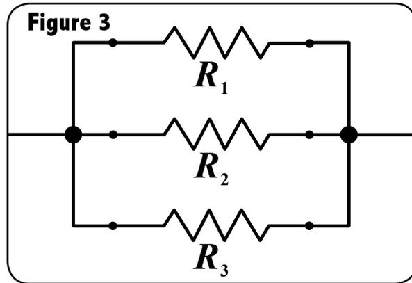
The sum of a set of parallel resistors is the reciprocal of the sum of the reciprocals of the resistor values:
