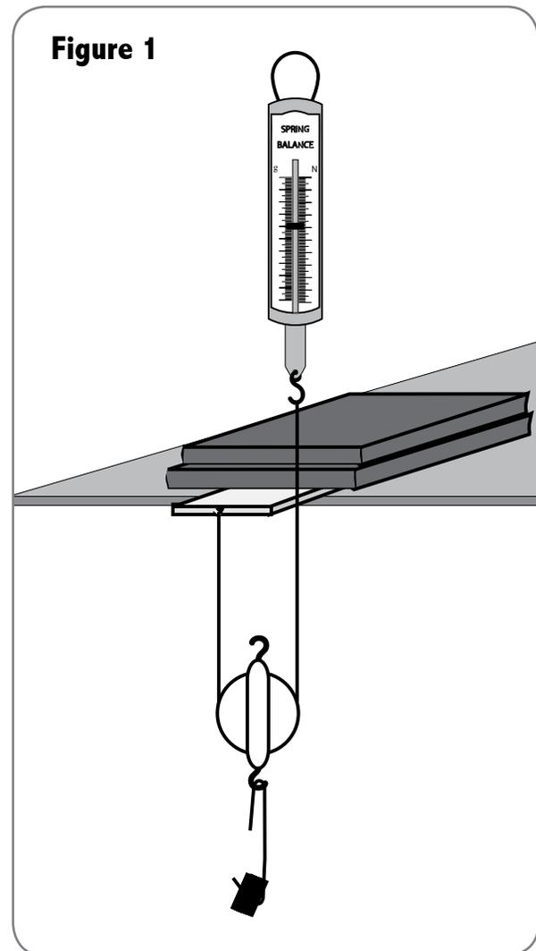
the force needed to hold the washers in position. The resistance force is the total weight of the five washers and the single pulley.
